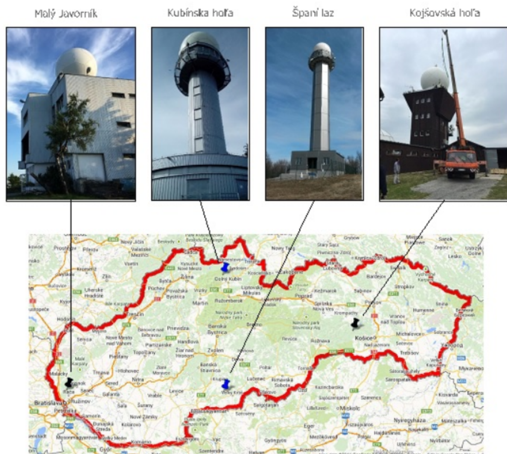
Figure 1.7: Slovak radars placement and appearance.
