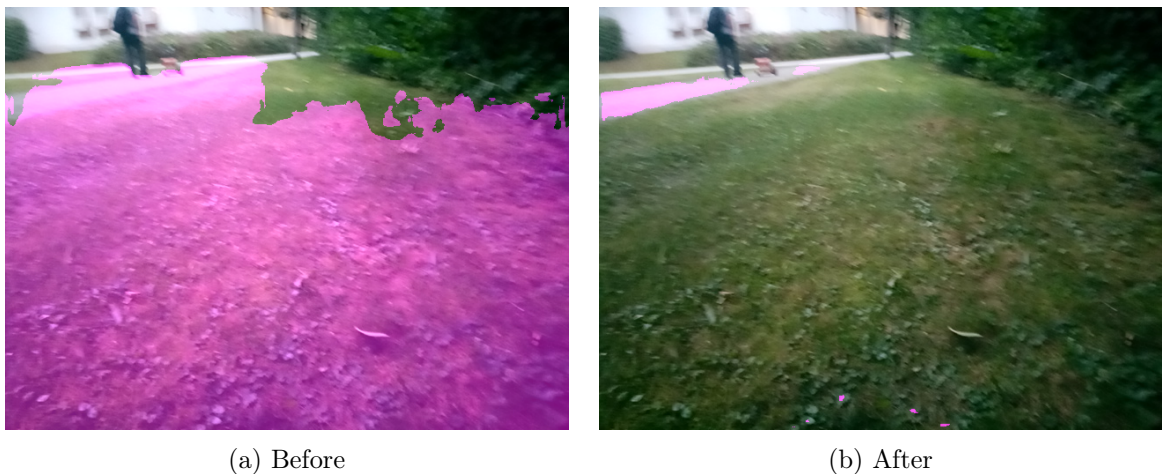
Figure 3.4: Predictions of images containing mostly grass. Image (a) shows the prediction before this kind of images have been added to the dataset while image (b) is the prediction after the dataset has been extended. Both images are predicted by the same ResNet. The only thing that has changed is dataset.
